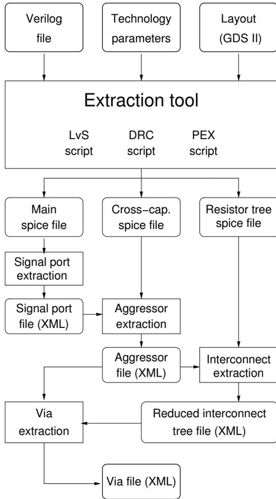
Figure 3: Parameter extraction flow
